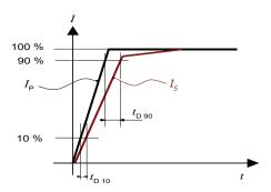
Figure 6:  $t_{\rm D\,10}$  (delay time @ 10 %) and  $t_{\rm D\,90}$  (delay time @ 90 %)
