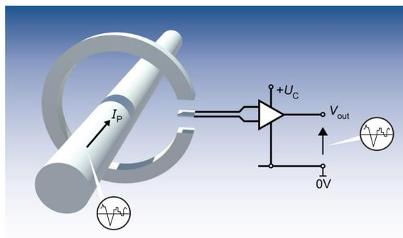
Fig. 1: Principle of the open loop transducer.
