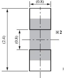
※2: Please note no short-circuit when the wiring pattern is arranged between the soldering attachment pad.
