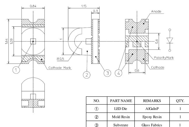
Note: The cutting burr size of the Print Circuit Board and Electrode isn't contained in the size of the height of the product.
