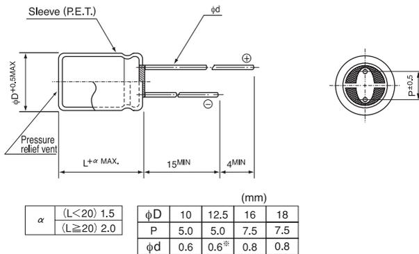
※ In case L > 25 for the φ12.5 dia. unit, lead dia. φ d = 0.8mm.
