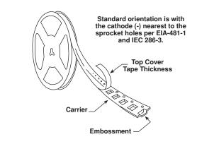
Tape and Reel Specifications: All case codes are available on plastic embossed tape per EIA-481-1. Tape reeling per IEC 286-3 is also available. Standard reel diameter is 13" [330mm]. 7" [178mm] reels are available.
