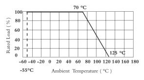
For temperatures in excess of  $70^{\circ}$ C the load shall be derated in accordance with the following figure.
