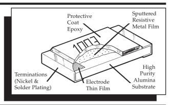
The RN73 series is a high stablity precision chip resistor range offering various power dissipation relating to chip size, TCR's down to 5ppm/°C and resistor tolerances to 0.1%. The resistor is produced with three sputtered layers giving better performance. Values are restricted to the E96 and E24 value grids. The RN73 has accurate and uniform physical dimensions to facilitate placement. They are of course packaged on tape and reeled.
