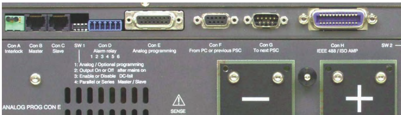
fig. 3 - 8 Location of output terminals and analog prog. connector on rear panel
