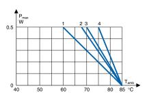
Maximum allowable power dissipation vs ambient temperature and case sizes.
