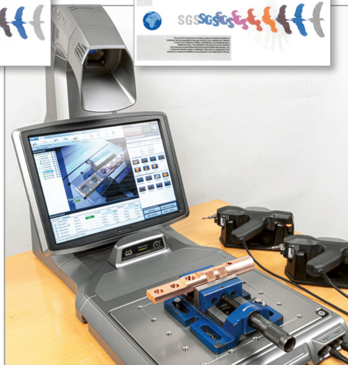
Opto-electronic measurement of the dimensions
