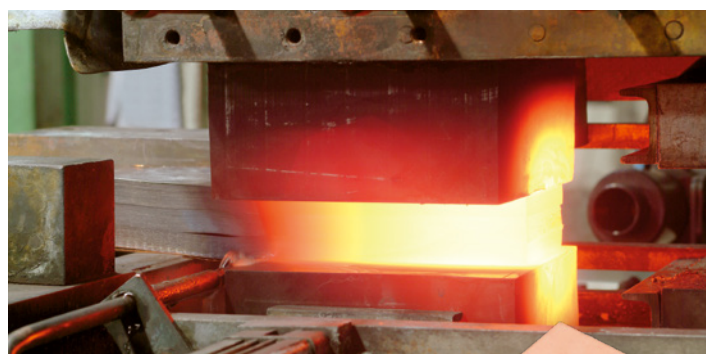
Pressure welding process for copper connectors
