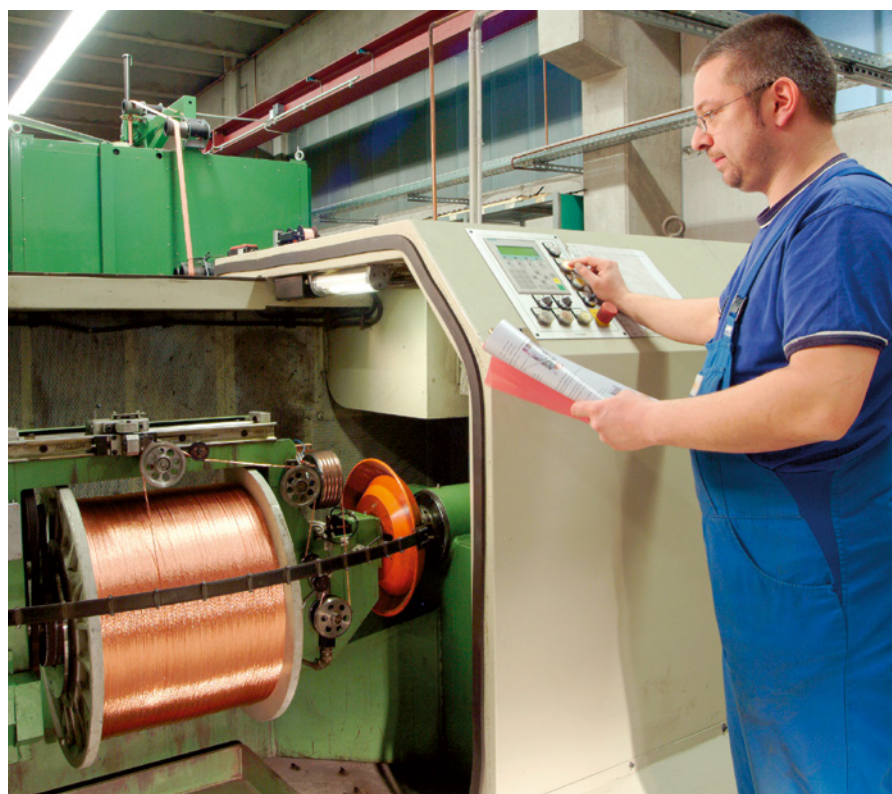
Twisting and stranding of highly flexible conductors
