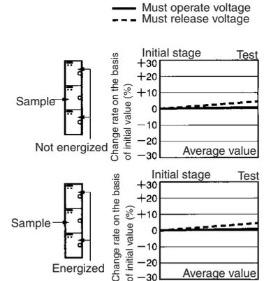
**Note 1:** The test was conducted at an ambient temperature of 23°C.
