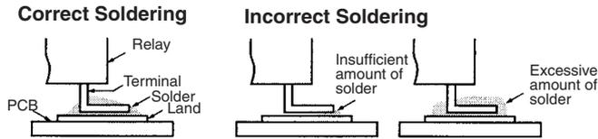
Visually check that the Relay is properly soldered.
