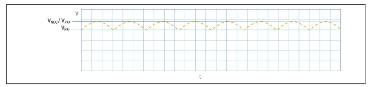
The applied peak-to-peak ripple voltage shall not exceed 0.2 x  $V_{\text{NDC}}$ . The peak voltage shall not exceed the rated voltage  $V_{\text{NDC}}$ .
