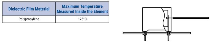
Temperature monitored inside the capacitor.
