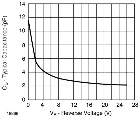
Figure 2. Diode Capacitance vs. Reverse Voltage  $V_R$
