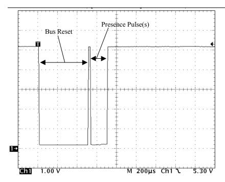
This image also shows a bus reset/presence sequence. The master pulls the bus low for 480 us, which is longer than any time slot can hold the bus low. All the devices on the bus recognize this as a Reset operation. Slave devices respond to a Bus Reset by issuing a Presence Pulse. Multiple slaves will generate their presence pulses during the same period, and they will overlap to form a single pulse. (Note that the time base is 200us per division.)
