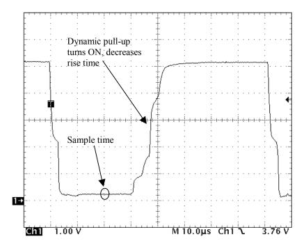
Here is the same dynamic pull-up operation in a Read Zero time slot.
