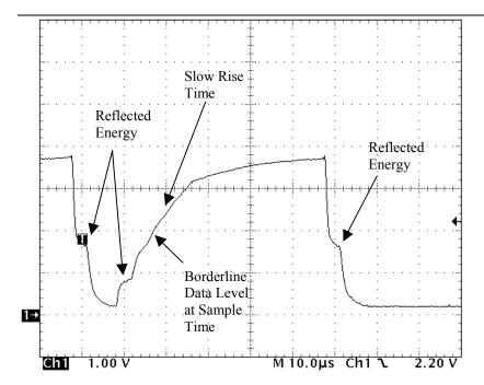
This image shows the effect of excessive weight when using a master with resistor pull-up only. The network radius in this example is 1000 feet and there are 30 devices at the far end of the network. The reflections from the end of the network can be clearly seen, as can the very slow rise time. Note that although this is a Read One time slot, the data level at the sample time is borderline and could be misread by the master.
