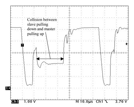
This image shows the resulting chaos that occurs when the dynamic pull-up is falsely triggered by reflections on the cable due to stubs and branches. This is a Read Zero time slot, although the reflection has caused the dynamic pull-up to activate and collide with the pull-down in the slave device.
