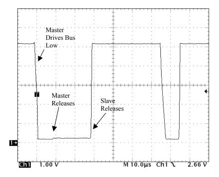
This image shows a "Read Zero" time slot. The master pulls the bus low for about 10 us and then releases it. However, a slave device is returning a zero bit by holding the bus low for a longer time. The slave device time base may vary between 22 and 60 microseconds. The master samples the bus at 20 us and so reads a zero bit in this example.
