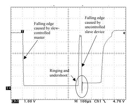
This image shows a Bus Reset and Presence sequence, but more importantly it shows the difference between the behavior of the slew-rate controlled master and the uncontrolled slave device. The falling edge created by the master is clean and does not undershoot or ring. The falling edge caused by the slave device is uncontrolled, and it can be observed to cause ringing and undershoot on the bus.
