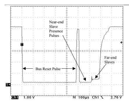
During Bus Reset sequences, the dynamic pull-up is used to overcome the network weight after the reset pulse, and then again after the end of the presence pulse(s). In this image, the overlap of near- and far-end presence pulses can be observed. The added resistance of the cable between the master and the far-end slave causes the low level to be higher for far-end devices than for near-end devices.
