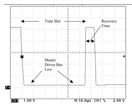
This image shows a "Write Zero" time slot. The master pulls the bus low for 60 us and then releases it for about 10us before another time slot begins.
