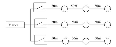
The example above has the appearance of a star topology network with a radius of 150m and a weight of 450m. However, when each switched path is considered one-at-a-time, the network is actually a linear topology and the weight is only 150m.
