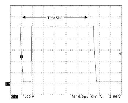
This image shows a "Read One" or "Write One" time slot. The master pulls the bus low for about 10 us and then releases it. Note the slew-rate controlled fall time. The time slot lasts for about 70 us, after which another time slot occurs. (Note that the time base is changed to 10us per division.)
